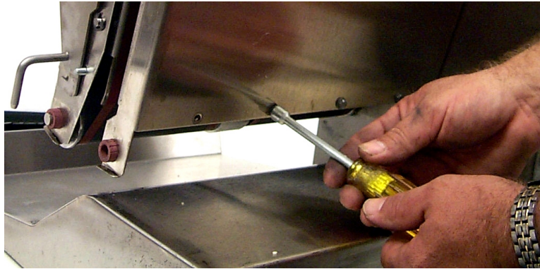
Remove screws securing platen to toaster conveyor assembly.
